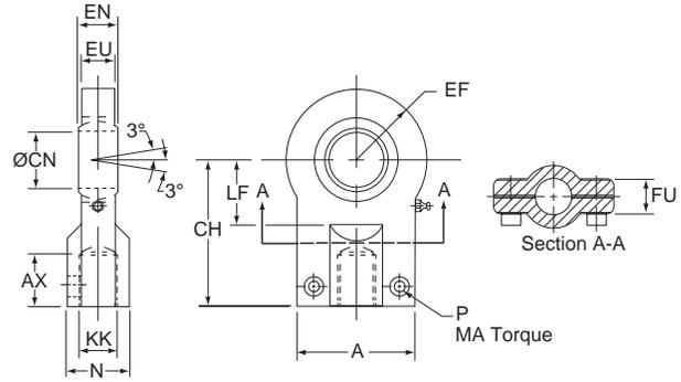
**Rod Eye with Spherical Bearing**
