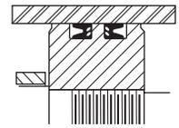
Standard on 50mm bore sizes and larger, B style piston is a single seal design which incorporates two wear strips. This design provides smooth operation, long bearing life, and high load carrying capacity.
