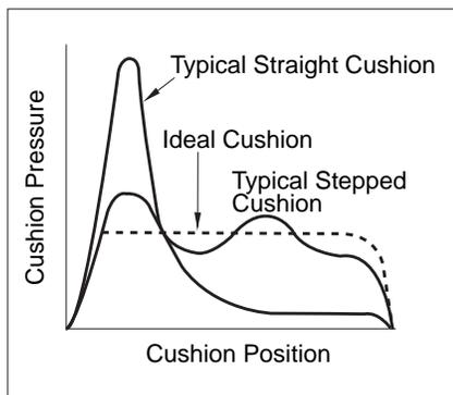
In order to cover the majority of applications, HMI cylinders are supplied with profiled cushioning as standard. Final speed may be adjusted using the cushion screws. The performance of profiled cushioning is indicated on the diagram, and cushion performance for
