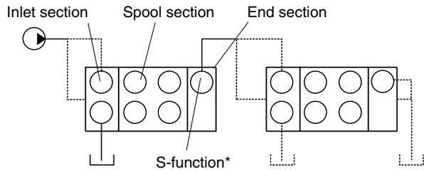
If an additional pump is connected to valve 2, then valve 2 receives the flow from pump 2 plus any residual flow from valve 1.
