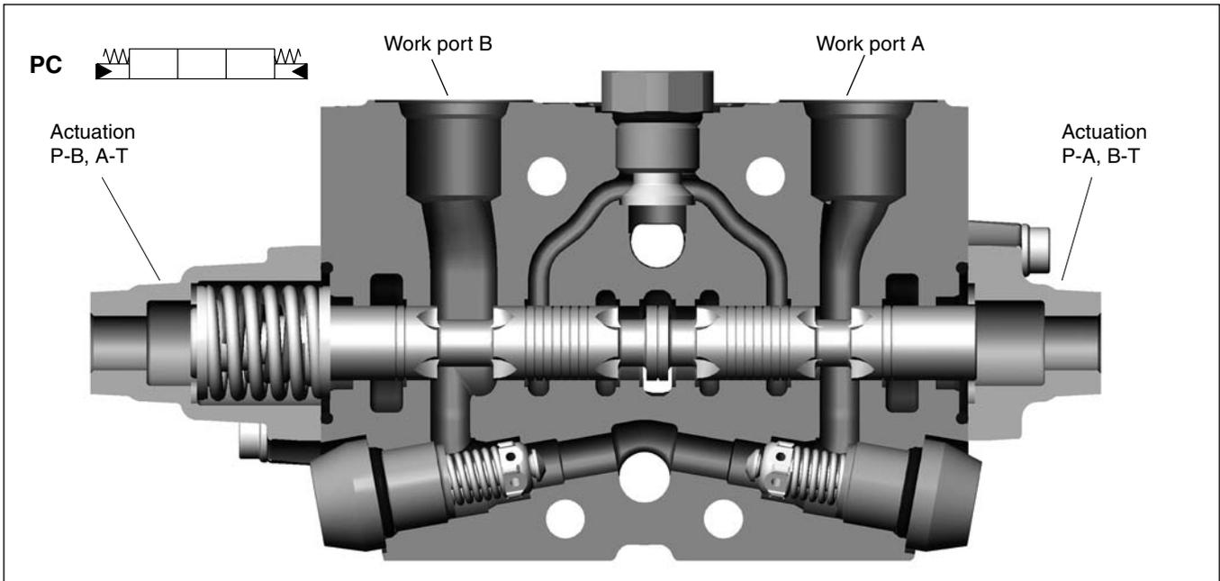
**PC** Hydraulic, proportionally controlled, spring-centred spool actuator. Best controlled by PCL4 remote control valve (see separate brochure).
