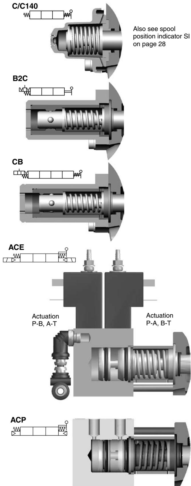
**Remote controlled proportional spool actuators with closed spool end**
