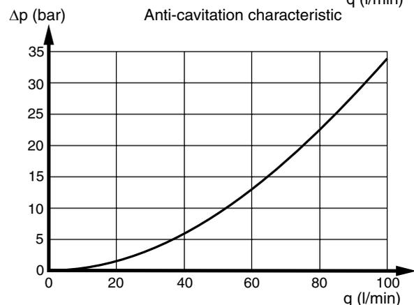
The curve shows the pressure drop between the tank connection and work port when port relief valve (PA) or anti-cavitation valve (N2) without port-relief function is used as an anti-cavitation valve.
