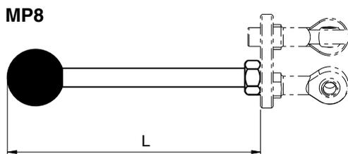
**Hand levers for closed spool-actuators**
