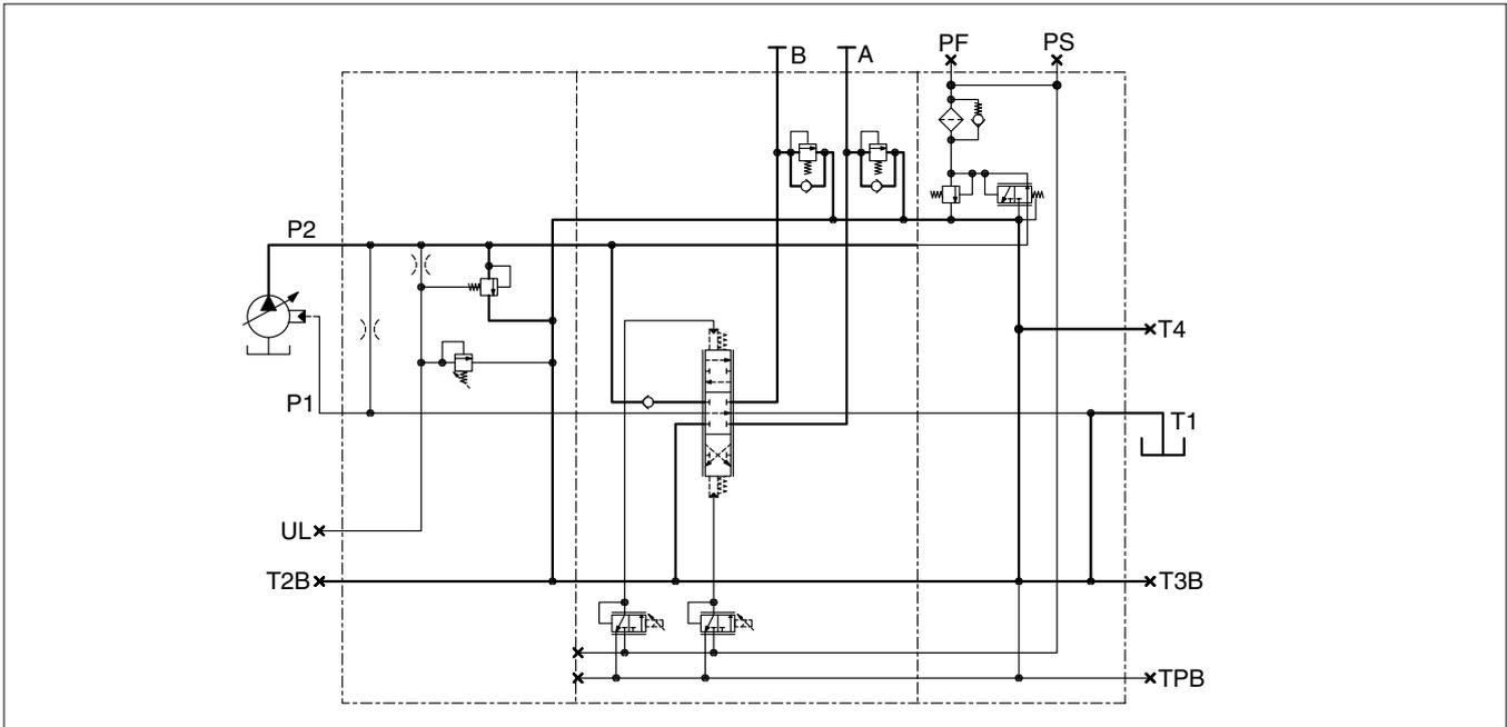
Principle circuit diagram for valve with closed centre
