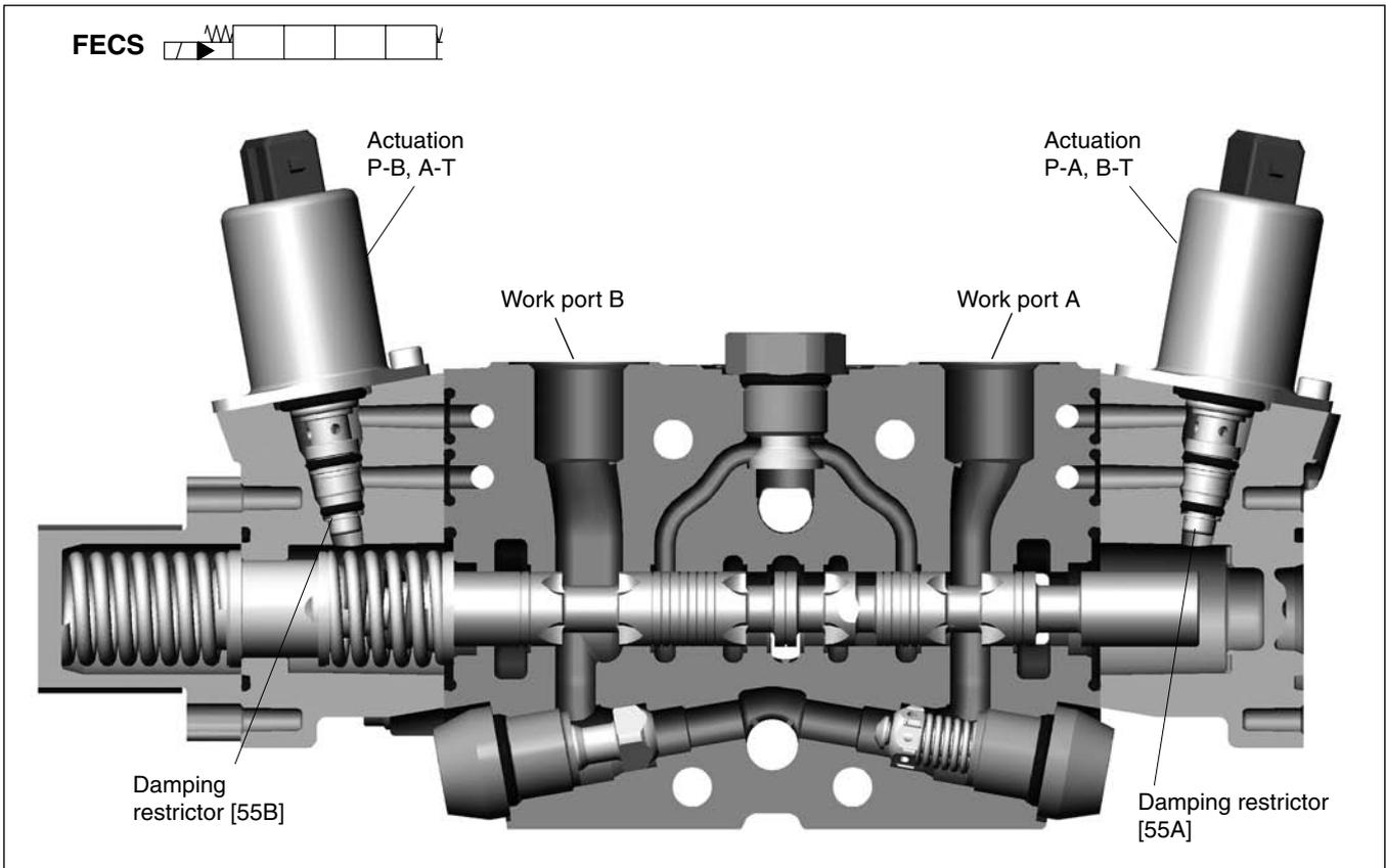
**FECS** Electro-hydraulic, proportionally controlled, spring-centered spool actuator with a fourth position for shifting the spool into the float position. The PS25 cartridge valve is used as its remote control valve.
