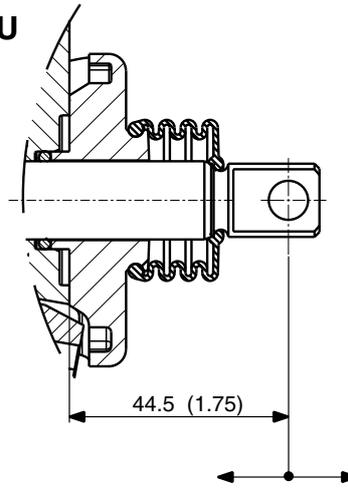
Spool stroke 12.5 mm (0.49) for spool function F [60]. Others 6.0 mm (0.24). Opens pump to work port A.
