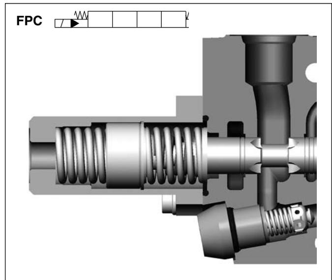
**Remote controlled proportional spool actuators with closed spool end
