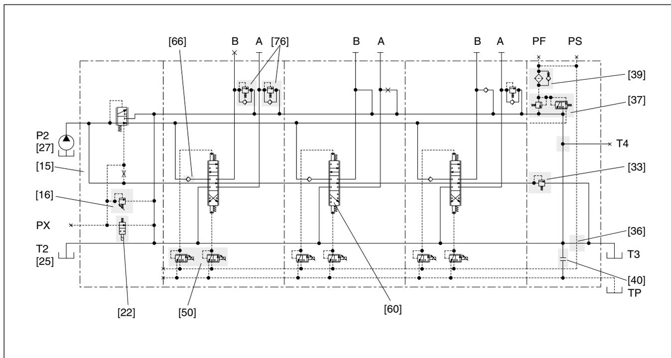
The circuit diagram above shows the P70 with three electro-hydraulically controlled spool sections and an integrated pilot-oil
