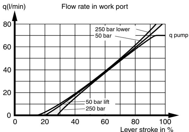
*In the P70CF equipped with FPC, PC, ECS and ECH closed spool-actuators, the spools are pressure compensated, with the result that the load's influence on speed is negligible.*
