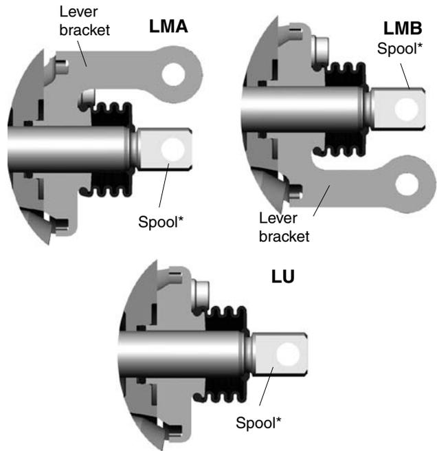
**MJA** Lever bracket and link parts for mechanical joystick, type A, and for open spool end. Lever bracket MJA have always to be selected in the left section and lever bracket MJ in the right section. Lever itself not included. Must be ordered separately (see page 33).
