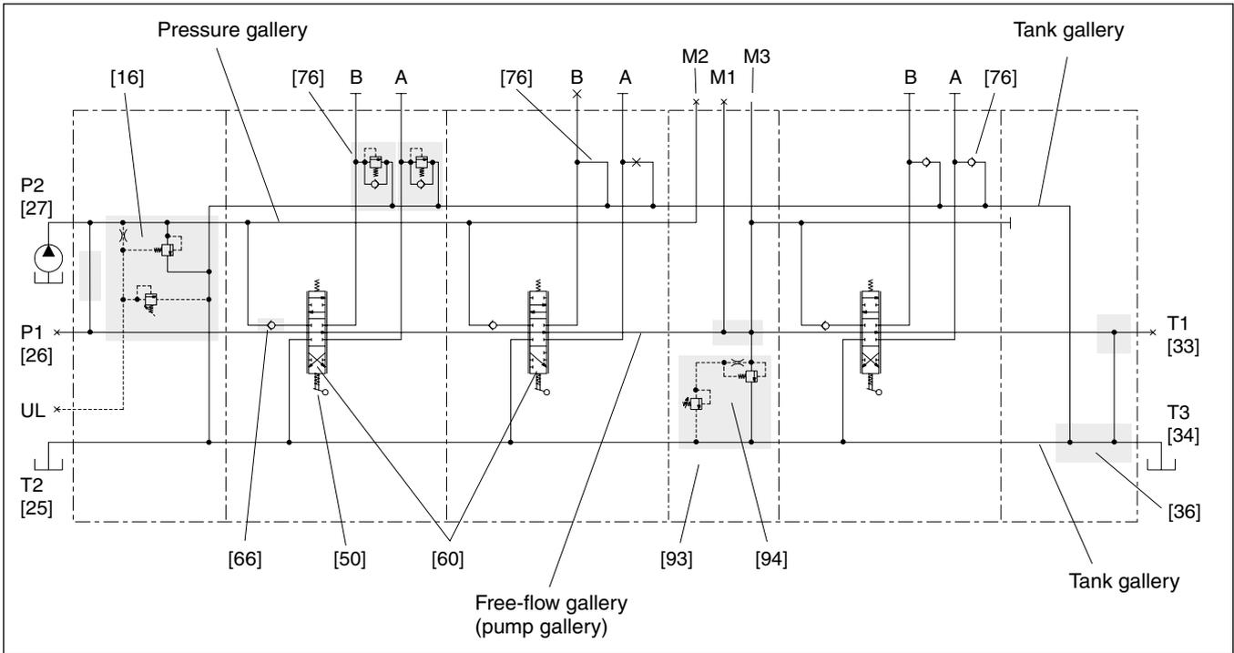
The circuit diagram above shows the P70CF with three spool sections and a mid-inlet between sections 2 and 3.
