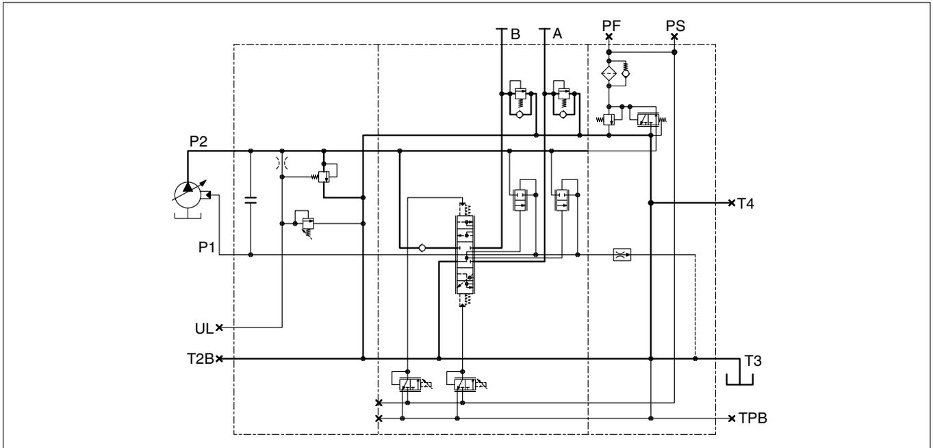
Principle circuit diagram for valve with load sensing
