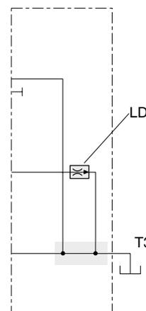
*Tank connection T3 open. Open centre gallery connected with tank through LD at item [33]. P70LS only.*
