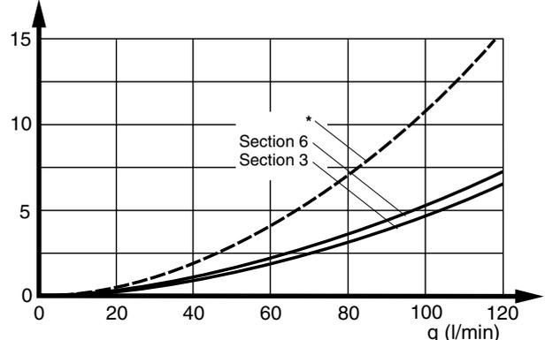
\* Broken line illustrates example of pressure drop in P70CF over a D-spool for q=65 l/min in section 6.
