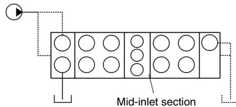
If an additional pump is connected to the mid-inlet section, then subsequent sections will receive the flow from pump 2 plus any flow from pump 1 that has not been used by the sections before the mid-inlet section.
