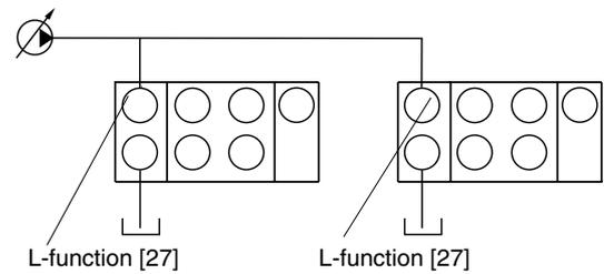
Parallel connection, variable pump (CPU, LS), P70CP, P70LS
